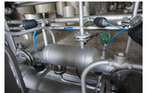
独立热交换器 Independent Heat Exchanger for precise temp control
